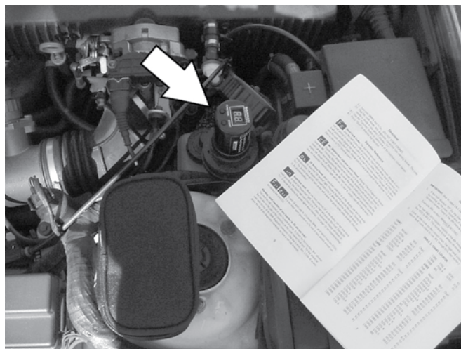
An affordable pocket-sized fault code reader plugged into the factory socket and the list of codes in the operator's manual.
