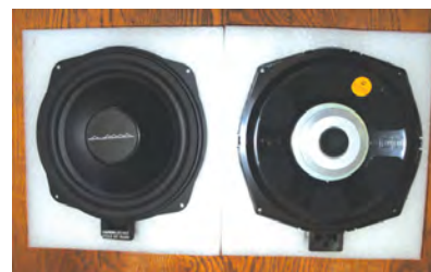
Identically sized. BAVSOUND speaker (L) and original OEM speaker (R).
