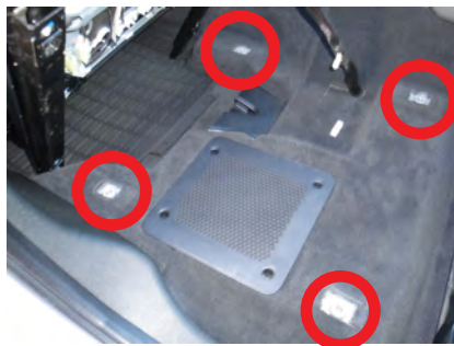
Speaker access couldn't have been more straight forward. Just four bolts to remove the seat.
